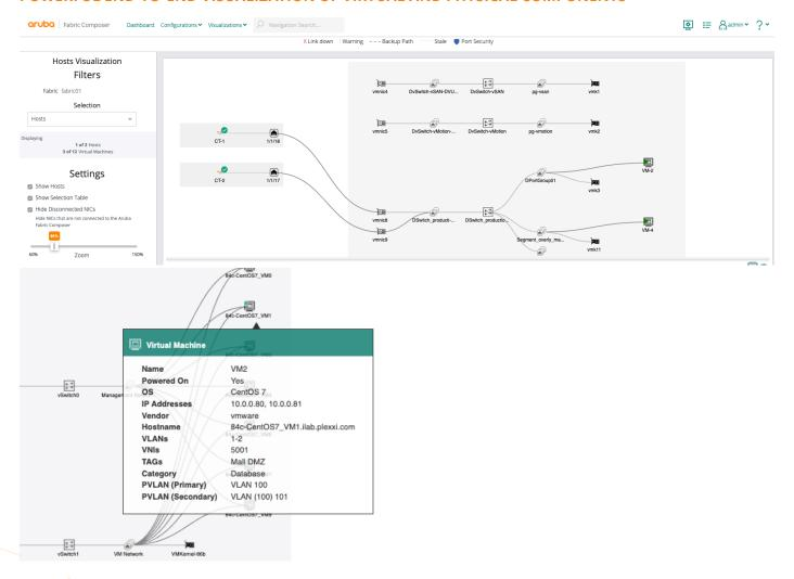
Using the Aruba Fabric Composer Host View, administrators can easily see end-to-end connectivity between Virtual Machines, Port Groups, vSwitches, and Physical NICs to visualize how they are connected to Aruba CX switch ports.
